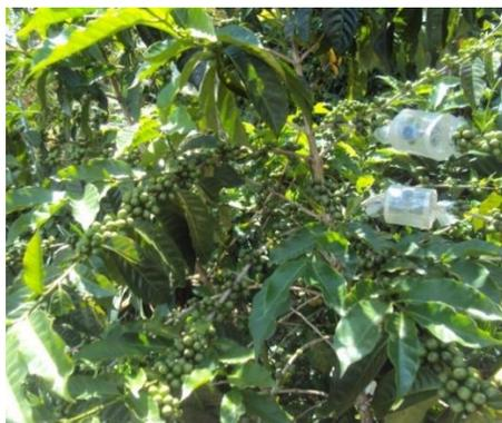
**Figure 1.1.** Cylinders ( $h = 8.1$  cm and  $r = 3$  cm) used to take samples of ethylene and  $\text{CO}_2$  produced by coffee fruits on plant in Tanetze de Zaragoza, Mexico.
